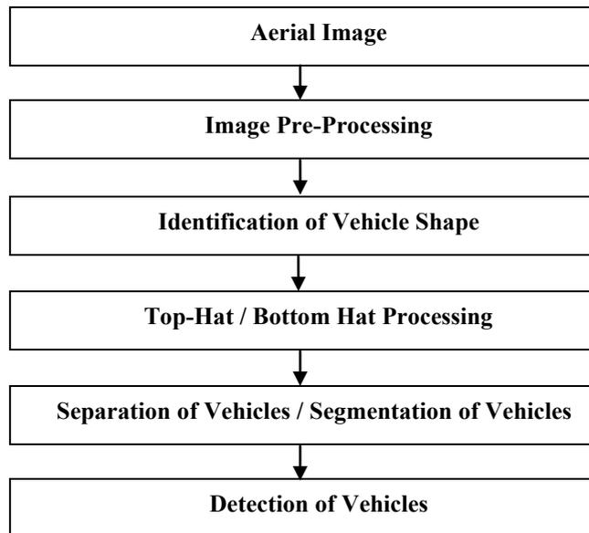
Figure. 1 Vehicle Detection Flowchart for TOP-HAT/Bottom Hat Operation.
