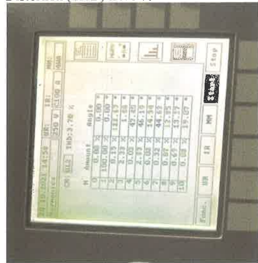
(ii) Phase 'b' voltage Total Harmonic Distortion (THD) :3.76 %
